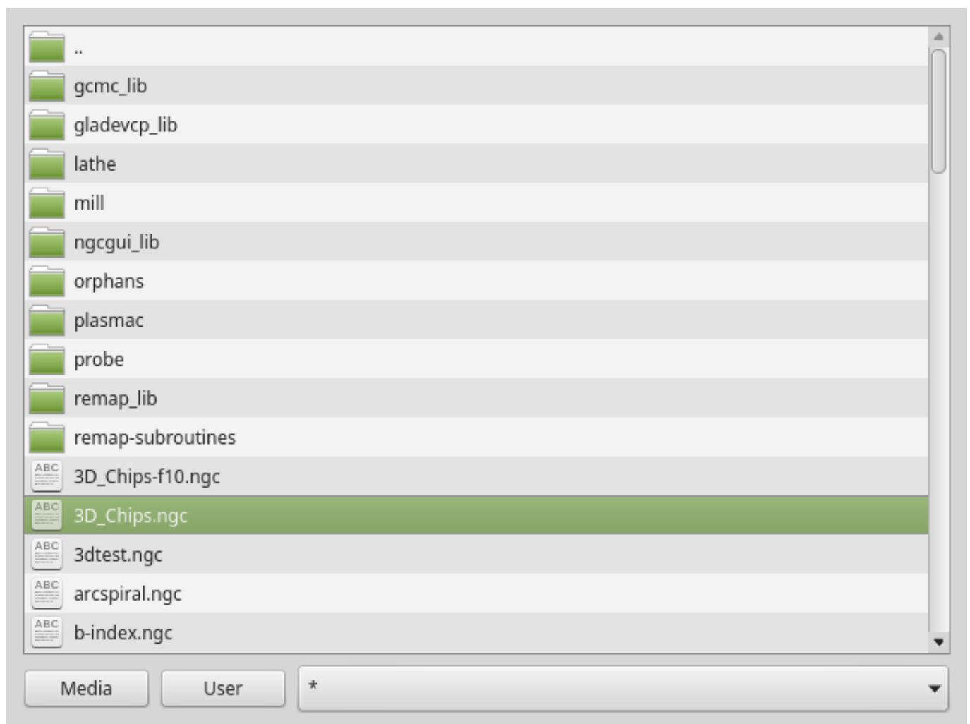
Figure 12.90: QtVCP FileManager: File Loading Selector Widget
