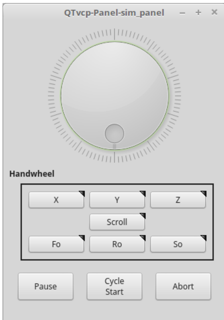
Figure 10.71 - QtVCP sim panel - Simulated controls for screen testing.
